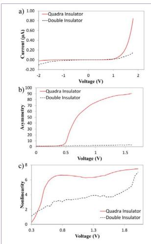
Figure 2: (a) Current – Voltage (I-V) curve (b) asymmetry (c) nonlinearity of the  $\rm Ml^2M$  and  $\rm Ml^4M$  diodes.
