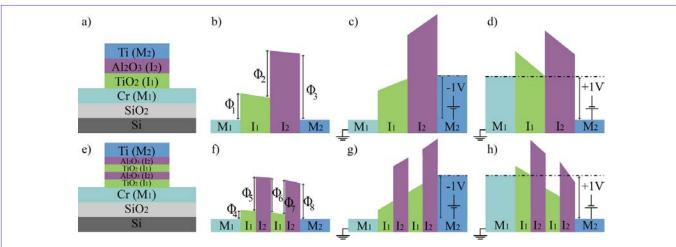
Figure 1: (a) A schematic diagrams of the cross-sectional view of the Ml²M diode. Energy band diagram of the Ml²M diode: (b) no bias applied; (c) negative; (d) positive bias applied to Ti; (e) A schematic diagrams of the cross-sectional view of the Ml⁴M diode. Energy band diagrams of the Ml4M diode; (f) no bias applied; (g) negative; (h) positive bias applied to Ti.
